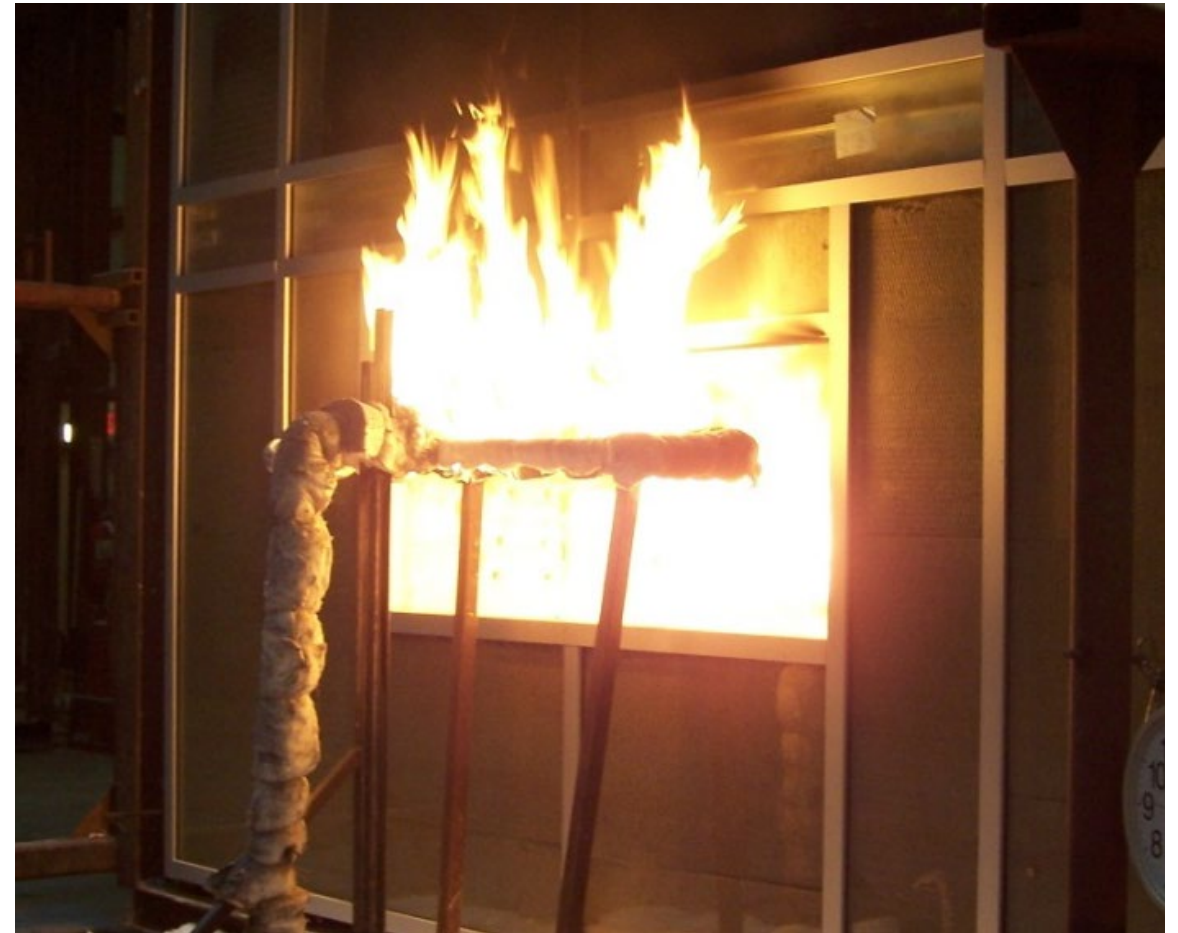
Perimeter fire barrier testing to E2307 – fire exposure from both below and from outside
